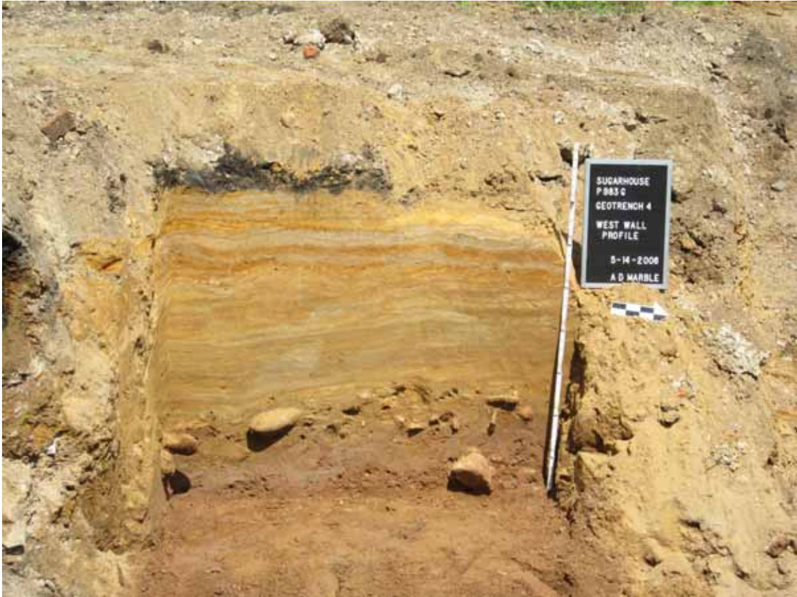
Figure 2. Closer view of the stratified recent alluvium atop the lower subsoil remnant of a truncated Coastal Plain soil. Each Band in the recent alluvium likely represents a single depositional event.
