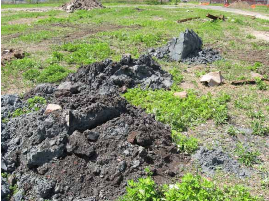
Figure 2. Dark gray, variably organic estuarine sediments excavated from beneath 11.5 feet of rubble fill in Trench SRT 2.
