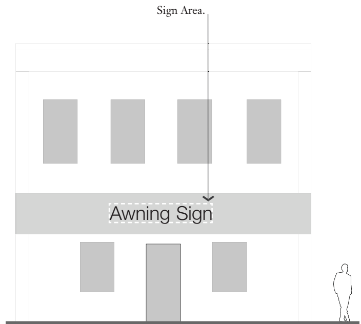
Figure 2.5-9(2). Measuring Awning Signs.
